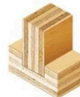
Set Accommodates Undersized Plywood
